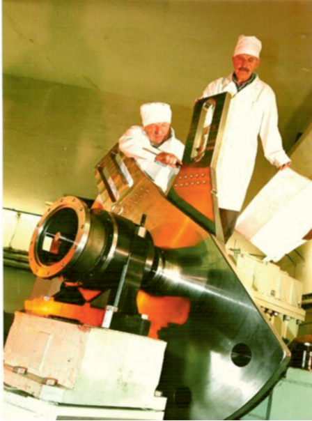
Figure 8. Movable reflector of the IBR-2 reactor.
